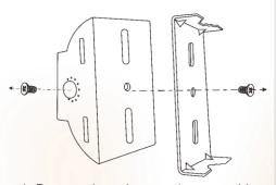
1, Remove the pole mounting assembly and CPE mounting arm.
