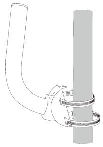
Insert the metal cable tie through the mounting hole and install it on the pole.
