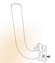
3, Install CPE mounting arm and adjust Angle.
