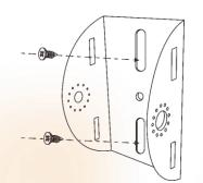
2, Nail the wall hanging assembly to the wall.
