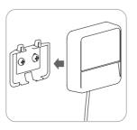
Mount the MHub Essential in a central location. For best coverage, we recommend mounting the MHub 160 cm from the floor.
